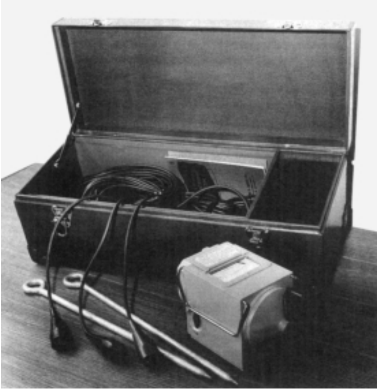
Figure 6-13. Megger Ground Tester.
