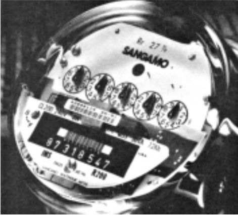
Figure 17-10a. Meter Equipped for Remote Reading by Radio.
